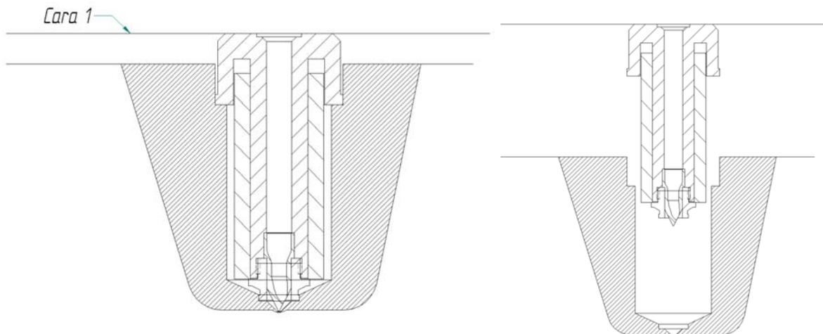
Nozzles must be centred on its position, with the utmost care taken not to damage them (C type is very delicate). A Cu washer must be placed on each nozzle head.
